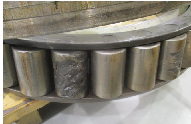
Figure 1: Screw compressor bearing rolling element defect
