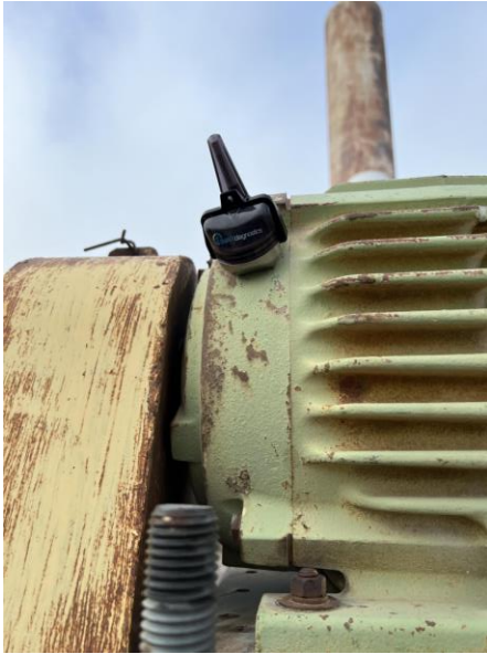
Above: Wireless, magnetic vibration sensor
