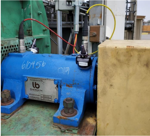
Figure 2: KCF's easily mounted magnetic, wireless V3 Sensors alongside an older style wired sensor that requires much more installation work and maintenance
