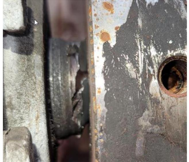
*Figure 1: A sheared drive shaft due to abrupt operating condition changes saved before further equipment damage was done.*
